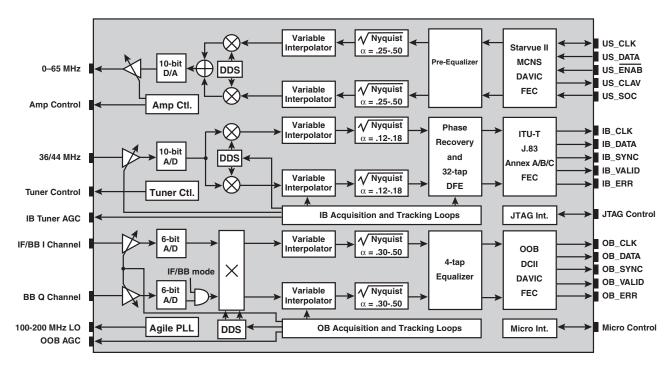
The Broadcom **BCM3125** combines an in-band 256-QAM receiver, an out-of-band QPSK receiver and a 4/16-QAM transmitter, providing an integrated set-top box or cable modem front-end solution.
